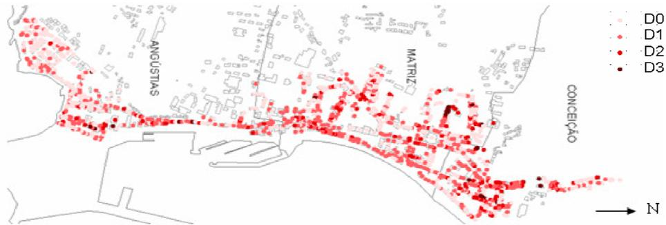
Figure 5: Damages occurred with Faial earthquake.
