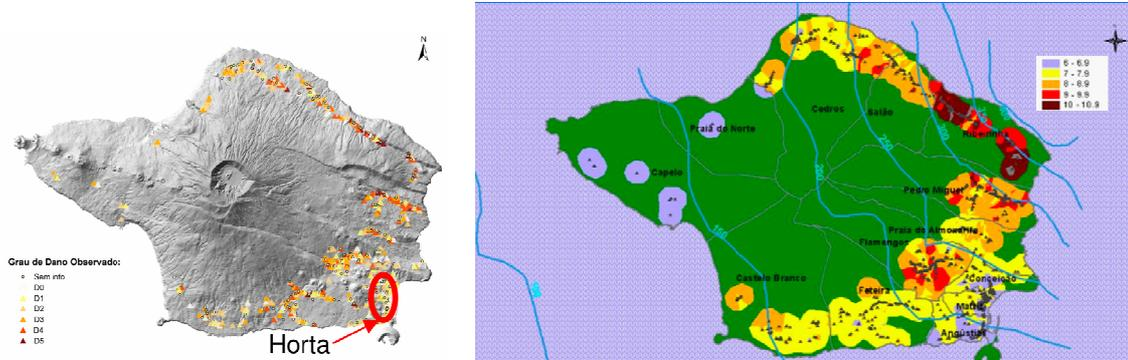
Figure 7: left – Real damage observed after 1998 earthquake (Ferreira, 2008) from "integrated data base". Right – *e-Risk*: Calculated intensities in Faial Island for the 1998 earthquake. Isoline in blue represents PGA ( $\text{cm/s}^2$ ); dots are buildings damaged; intensities were computed for urban areas with a radius of influence of 3 km. (see location of Horta).
